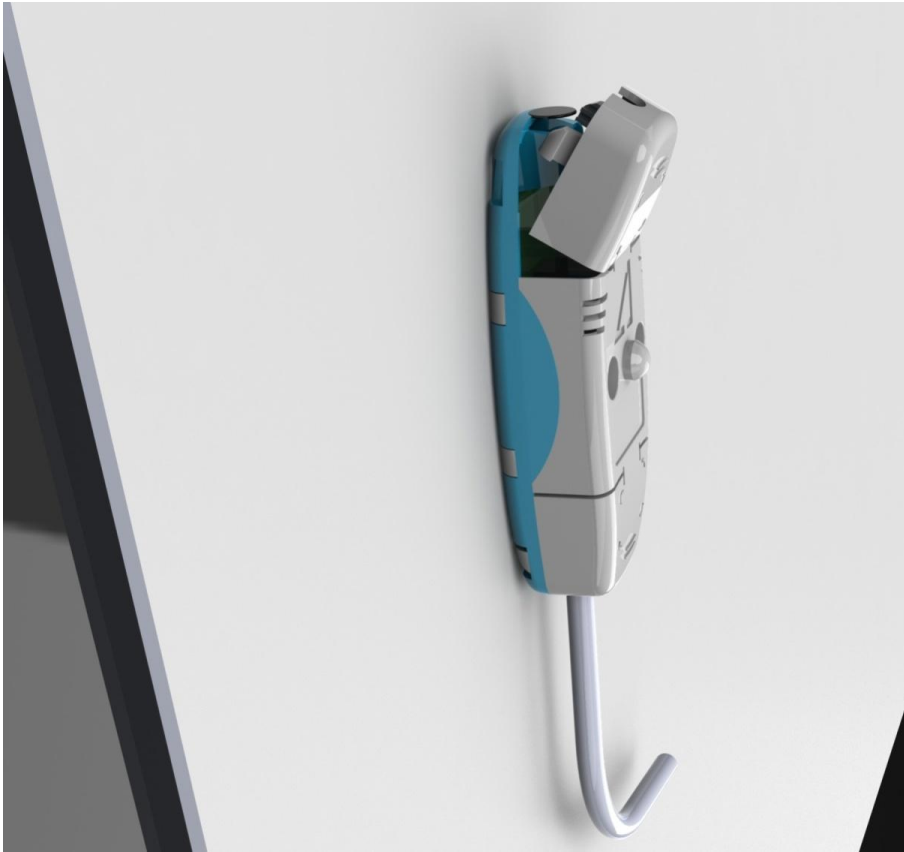
Figure 4-2: AQ 01 mounted to compartment wall.
