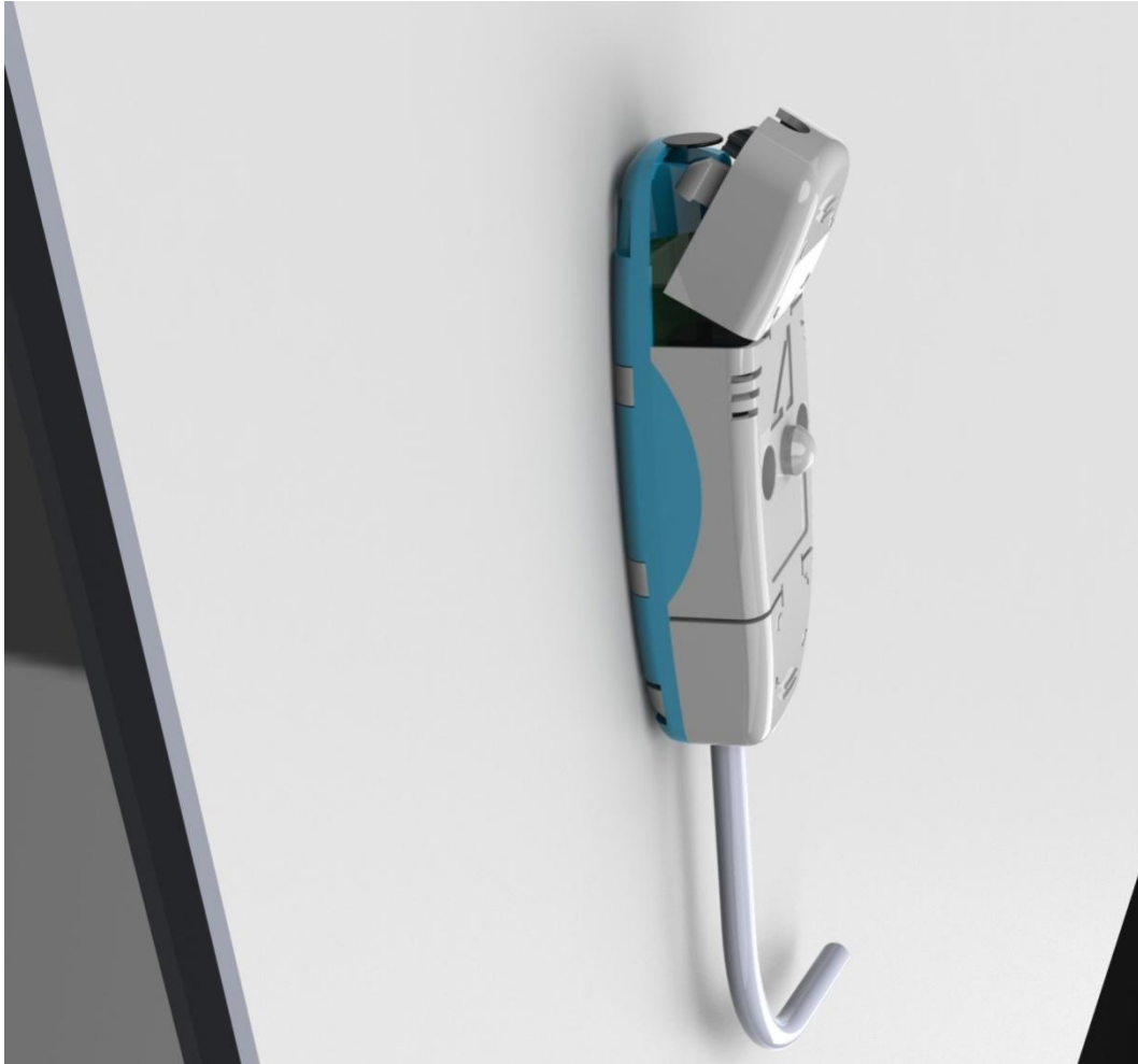
Figure 4-2: AQ 01 mounted to compartment wall.
