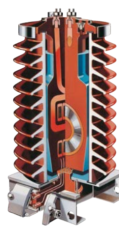
› Fig. 7. Current transformer; outdoor service; epoxy+porcelain
