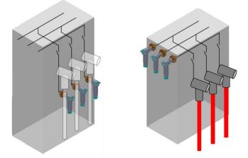
This redesign allows sending switchgear completely wired and tested from factory, avoiding wiring problems in installation, making it easier.
