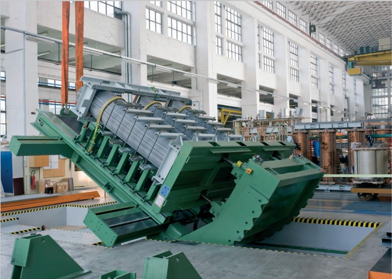
The lower yoke and the limbs are coated with glue varnish. Oscillations and vibrations caused by magnetostriction forces are thus reduced to minimum. The frame formed by yoke and limb clamps around the magnetic core enables safe transporting of the transformer and adequate resistance to electromagnetic short-circuit forces.
