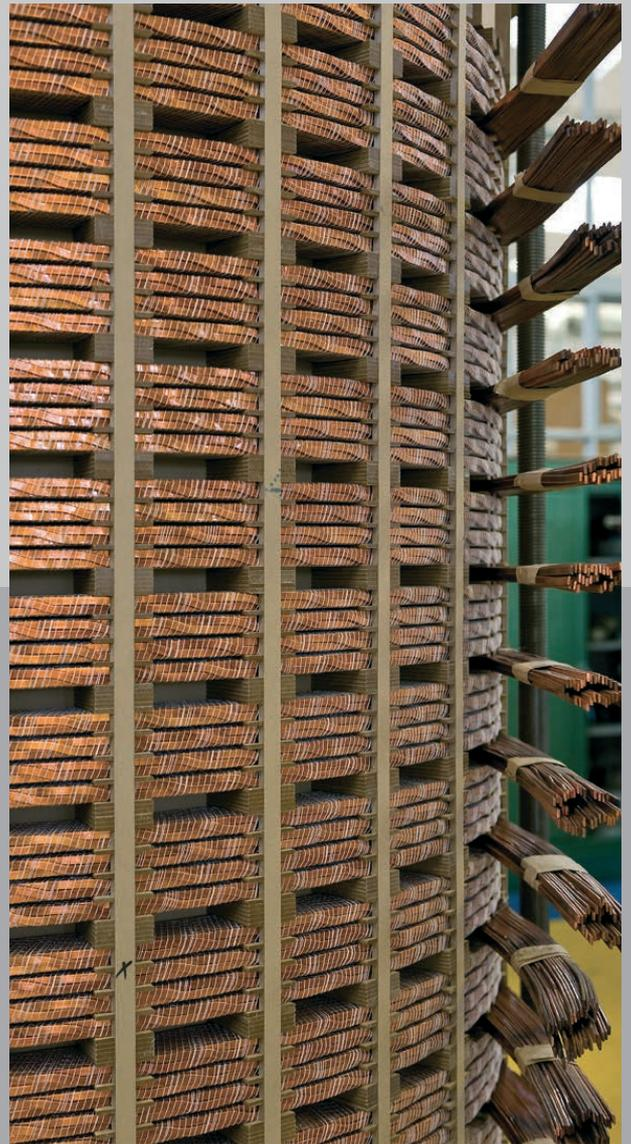
Plates and screws for longitudinal pressing of all windings for one phase and the radial tightening cylinder form a compact unit resistant to forces in case of eventual short circuit in the network
