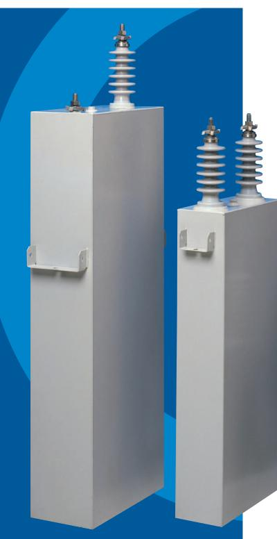
High voltage power capacitors are designed and manufactured by using latest technology and high quality materials. They have all-film dielectric and are impregnated with dielectric liquid which is biodegradable in environment. Each capacitor element has a separate internal fuse. In addition, each capacitor is provided with an internal discharge resistor.
