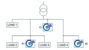
Figure 1: Installation of enclosed capacitor banks
